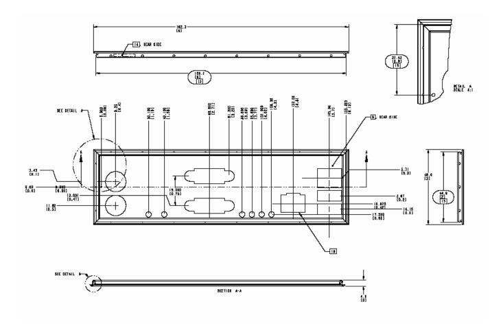
Figure 13. sku 2 Pedestal mount I/O shield mechanical drawing
